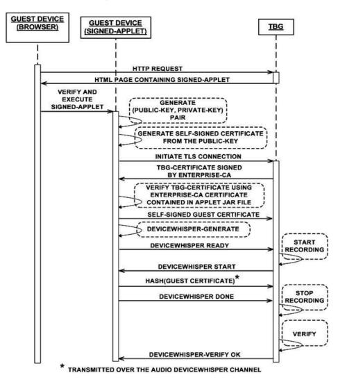
The recovered bits are then compared with the certificates obtained through TLS handshake and is verified. If both the certificates are same the device will get authenticated.
